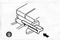
7 Pull the cable from the tool in a straight forward motion. Retract the cam wheel to remove any residual insulation. If the cut depths are not correct, repeat Steps 3 through 7.
